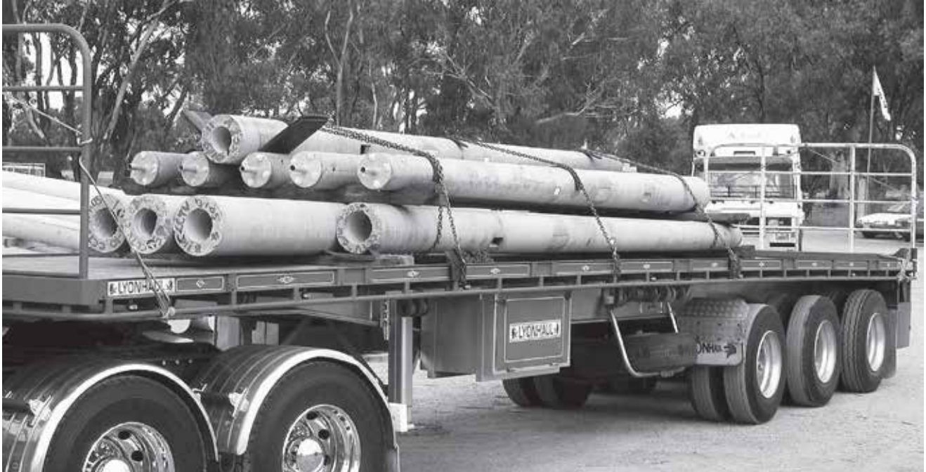
Longer poles should be placed on bottom layer
