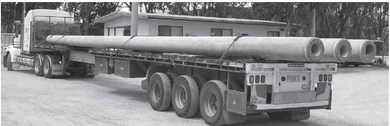
Use extendable trailer for poles or piles longer than 14m
