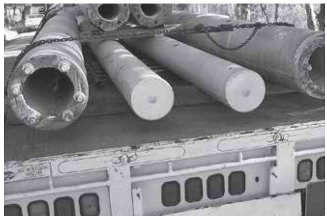
Poles of different diameters require support bearers and timber packing
