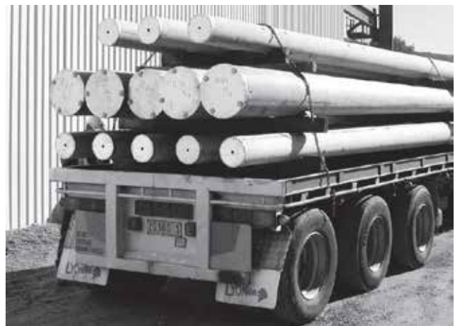
Poles with same tip diameter are placed together butt-to-butt
