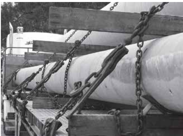
Poles or piles must not be secured via joint lugs
