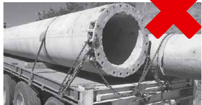
Poles or piles must not be secured via joint lugs
