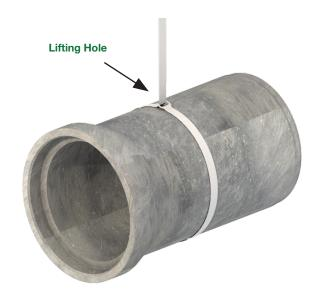
For pipes that do not have a lifting hole or where a sling is preferred, a belly sling can be used to lift and handle the pipes. Larger pipes can use one belly sling while smaller diameter pipes may use two for better handling. Whether one or two slings are used, adjust the position to ensure that the pipe is hanging horizontally.
