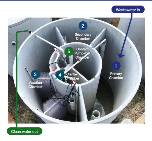
Now quite clear, the water enters the clarifier chamber where the remaining sludge from top and bottom surface is collected and returned to the primary chamber. This flows into the pump-out chamber where crystal clear water exits the system via a chlorinator and disinfector unit, through a high quality pump, and becomes available for irrigation.
